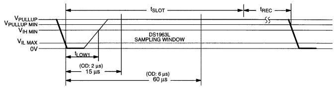
$\begin{array}{l} \mbox{Regular Speed} \\ 60 \ \mbox{$\mu$s$} \le t_{SLOT} < 120 \ \mbox{$\mu$s$} \\ 1 \ \mbox{$\mu$s$} \le t_{LOW1} < 15 \ \mbox{$\mu$s$} \\ 1 \ \mbox{$\mu$s$} \le t_{REC} < \infty \end{array}$
